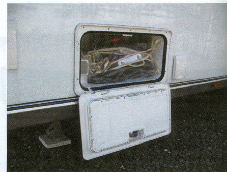
Wet locker which comes in handy and also houses the 13 amp socket for outside use.
