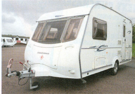
Two-piece aluminium sidewalls and ABS end panels make up the Amara's bodyshell BELOW The bed is made up as in the Swift, but the seat slats appear to be less durable
