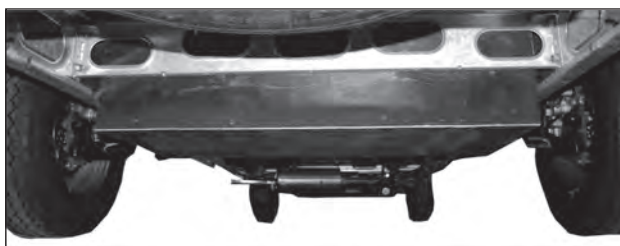
The grey water tank is mounted close to the motorhome's rear axle.
