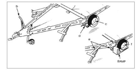
ALWAYS USE THE CORRECT BOLTS TO SECURE THE WHEEL, THERE ARE UNIQUE BOLTS FOR ALLOY WHEELS AND UNDER NO CIRCUMSTANCES SHOULD ANY OTHER BOLTS BE USED WITH ALLOY WHEELS.
