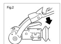
coupled to your towball) then the front/ rear friction pads, coupling ball and mechanism are in order.
