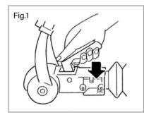
Press the red stabilising lever down. The AKS is now ready for the road. (Fig. 2)
