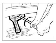
It is important that the caravan is correctly levelled to ensure the correct working of the refrigerator, cooker etc.
