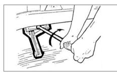
It is important that the caravan is correctly levelled to ensure the correct working of the refrigerator, cooker etc.
