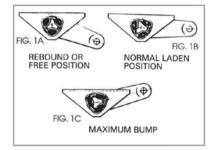
Three rubber elements are contained within a hexagonal axle tube. These provide suspension and have inherent damping characteristics.
