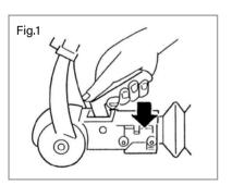
• Press the red stabilising lever down. The AKS is now ready for the road. (Fig. 2)
